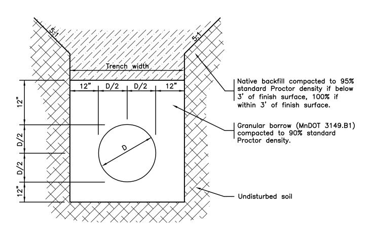
Note: Fill material shall be placed in 6" lifts or less and compacted to specified densities.
