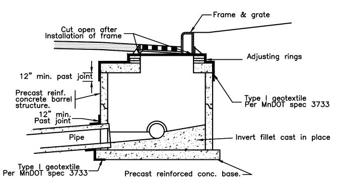
SEAL FABRIC ONTO CATCH BASIN AND CATCH BASIN MANHOLE WITH DUCT TAPE. OVER LAP ALL SEAMS. 12" MIN.
